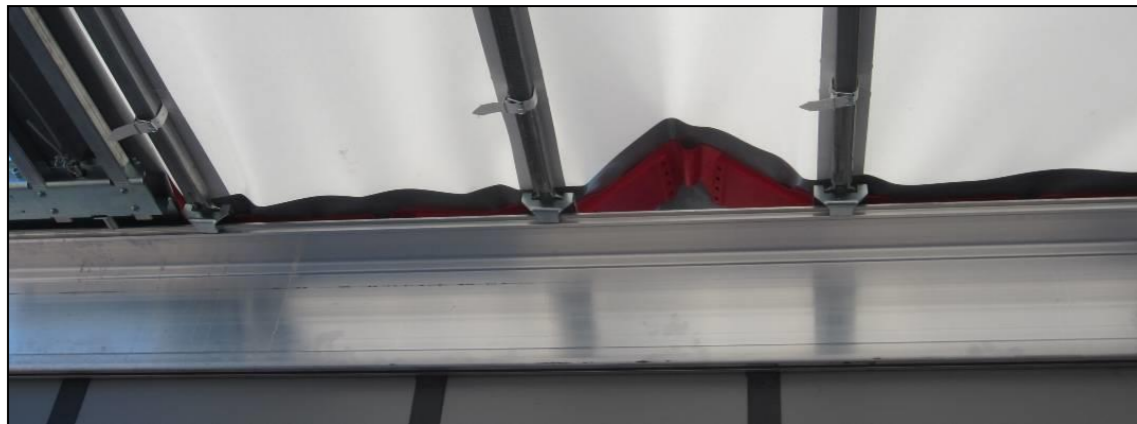
Dachaufsteller Versus (Spriegelabstand max. 570 mm Zollvorschrift) 22 Spriegel Versus Roof connectors (distance max. 570 between roofsticks) 22 cross roof cross members
