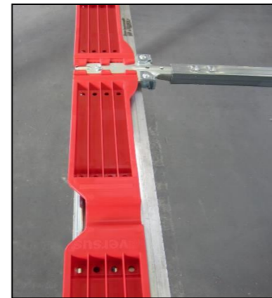
Dachaufsteller Versus (Spriegelabstand max. 570 mm Zollvorschrift) 22 Spriegel Versus Roof connectors (distance max. 570 between roofsticks) 22 cross roof cross members
